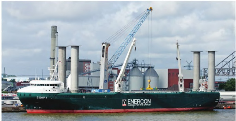
E-Ship1. Four large rotorsails rise from its deck to aid the ship's propulsion by means of the Magnus effect [the perpendicular force that is exerted on a spinning body moving through a fluid stream].
